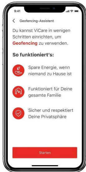
Image 2: Viessmann's ViCare app can use the smartphone location function and recognize the distance to the heating system if desired (geofencing). It will then automatically lower the heat output if nobody is home (available soon).
